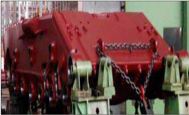
T-72 Hull Under Manufacturing
