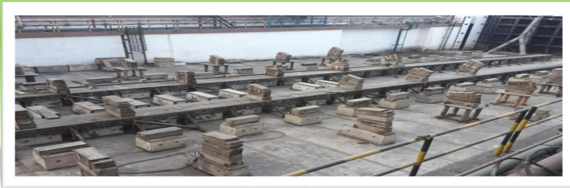
Dock block arrangement on inclined floor for 2 FPVs utilizing existing ground ways
