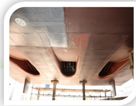
Dock block arrangement on inclined floor for 2 FPVs utilizing existing ground ways
