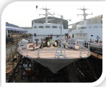
Dock block arrangement on inclined floor for 2 FPVs utilizing existing ground ways
